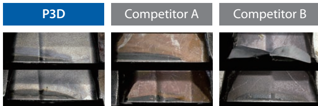
Wear comparison after drilling 48 holes
