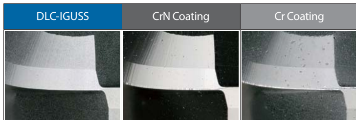
Wear condition of ball flank after milling 420m
