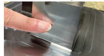
Finished surface by PFB-BR
