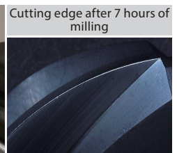
Cutting edge had normal wear without abnormal damage after finishing 7 hours of machining. Finished surface was much smoother and consistant versus competition.
